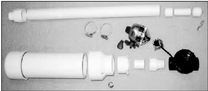
Figure 4 — The spudgun is easy to fabricate from the pieces shown.
