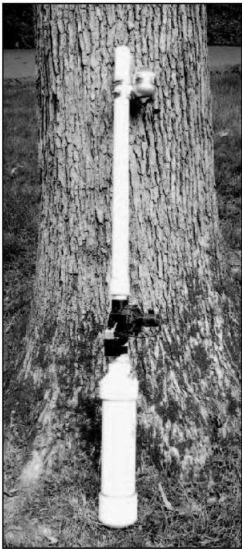
Figure 1 — The assembled antenna launcher ready to be pumped up and used.
